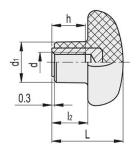
$\begin{array}{lll} D & = 50 \\ D1 & = 19 \\ DH & = M10 \\ h & = 17 \\ I2 & = 15 \\ L & = 30 \\ Weight in (g) = 37 \end{array}$
